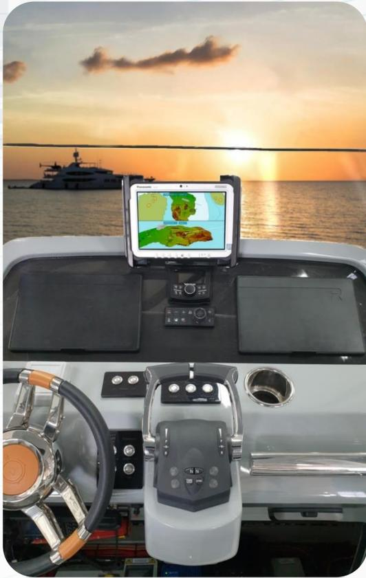
Wireless Tablet PC mounted at console
